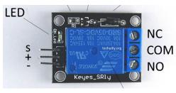
+ = 5V, - = Ground, S = signal (GPIO) NO = Normally open – connect to opener
