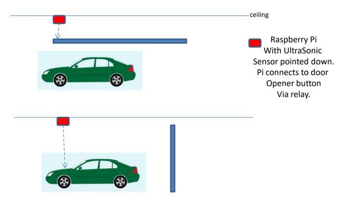
UltraSonic sensor gives distance to object, car present and door down, door up.
