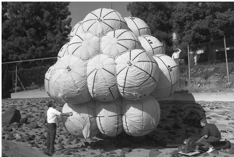
Figure 42-1: Cubic packing of the airbags on the Mars Pathfinder lander 1
