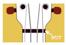
If you're experimenting with strings that are different from the ones your uke came with, make sure that they fit into the nut slots, because diameters may vary.
