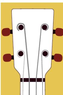
The two strings on the treble side of the instrument should wrap around the tuning pegs from the left, while the strings on the bass side should wrap from the right in order to ensure a straight string path.
