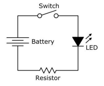
If no resistor LED would quickly burn out – most LED will take max of 25 mA and/or 1.7 to 2.1v (depends on color) before burning out!
