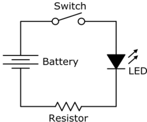
If no resistor LED would quickly burn out
