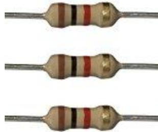
Type & physical size dependant on power to be consumed (as heat!) – typically we will be using ¼ Watt resistor shown on left.
