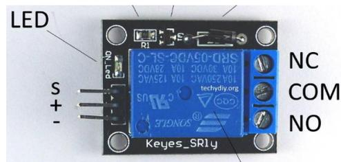
+ = 5V, - = Ground, S = signal (GPIO)
